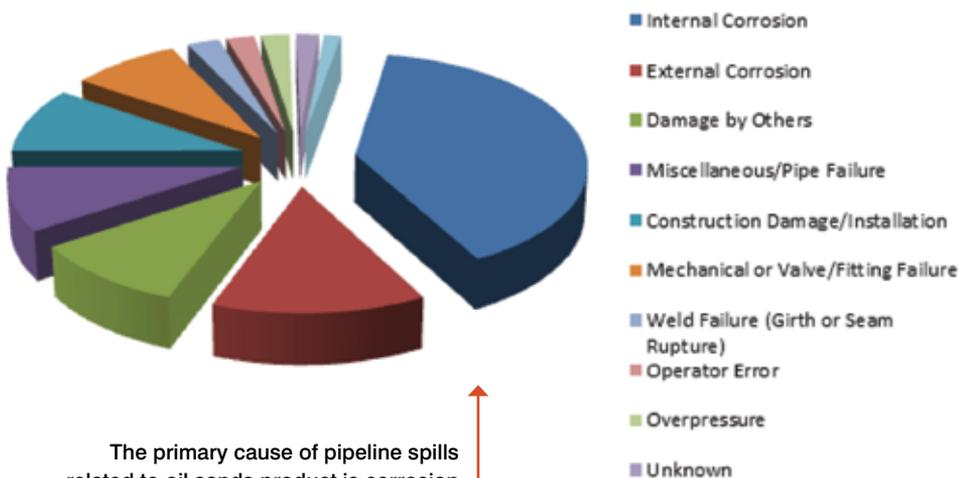
The primary cause of pipeline spills related to oil sands product is corrosion to the inner wall of the pipe (39 percent of all spills) and external corrosion of the outer wall (13 percent of all spills), according to data from the Canadian Association of Pipeline Producers ("Mitigation of External Corrosion on Buried Pipeline Systems," June 2009).
