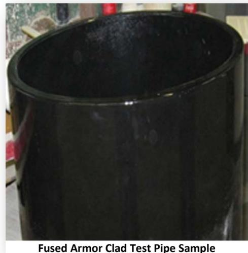
Fused Armor Clad Test Pipe Sample
